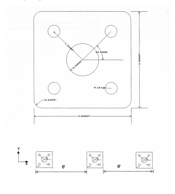
FIG. 1 Blueprint of flange part and the 3 fixtures.
