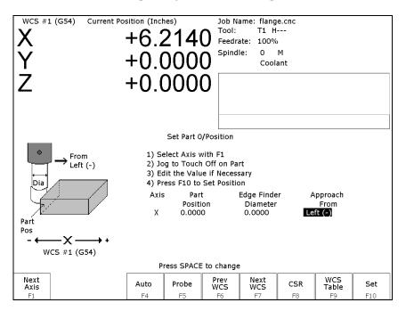
**NOTICE** Before manually jogging any probe, make sure the machine Feedrate is slow (less than 10 in/min) or damage to the probe may result!
