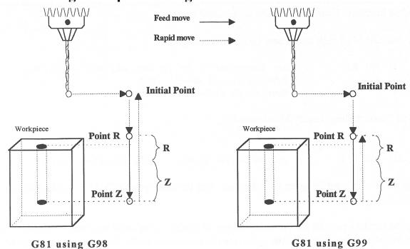
G81 is a general purpose drilling cycle. The hole is drilled in a single feedrate move, and then the tool is retracted at the rapid rate.
