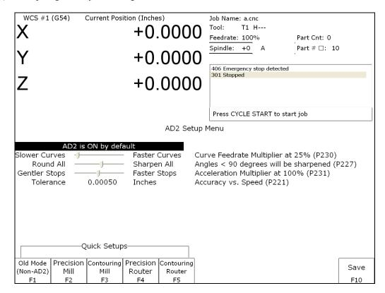
By default, AD2 will be turned off. The Quick Setup keys (F1-F5), will allow the machine to be configured to use AD2 (or not use AD2 in the case of F1). Start by selecting the most appropriate Quick Setup.
