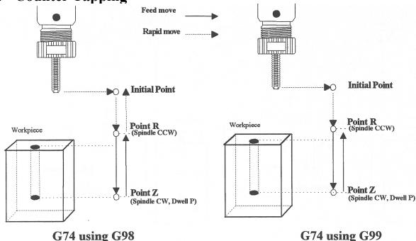
G74 performs left-hand tapping using a floating tap head. The spindle speed and feedrate should be set and the spindle started in the CCW direction before issuing G74. By default, G74 uses M3 to select spindle CW (at the bottom of the hole) and M4 to re-select spindle CCW (after backing out of the hole). Alternate M functions may be specified by setting parameters G74 (for CCW) and G84 (for CW).
