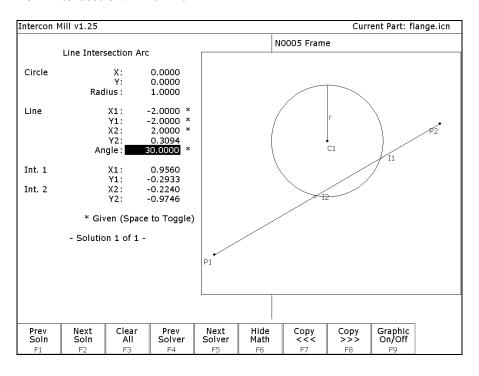
Given the center (C1) and radius (R) of an arc, 1 point (P1) and either a second point (P2) or one coordinate (P2 X or Y) and the angle from horizontal, find the intersection point(s) (I1 and I2).
