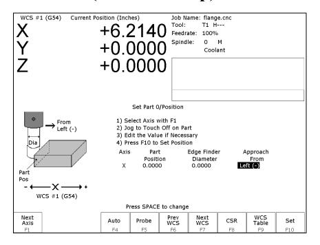
The Part Setup menu is used to set the part position or the coordinate system origin for the part.
