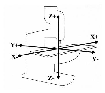
\*The direction of motion is defined by the CUTTER motion, not the TABLE motion.
