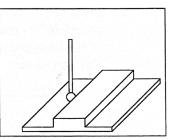
If the Z clearance you entered is too small, the probe will stop and show an error message. Correct the problem by repeating the previous steps. If the approximate width you entered is too small, the probe will bounce by 10 percent of its width across the top surface until it either finds the correct edge, the additional distance searched is equal to Parameter 16, or a travel limit is reached.
