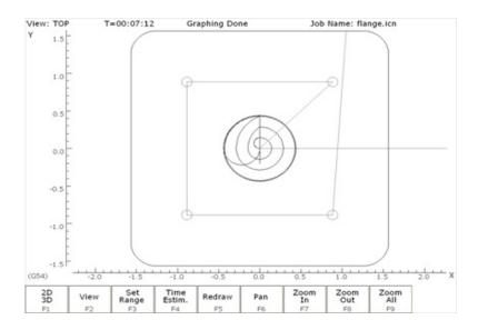
F1 - 2D/3D Press this key to view your part isometrically (3D). An axis pointer indicates the current direction of the view. To return back to the tri-planar view, press F1 again.
