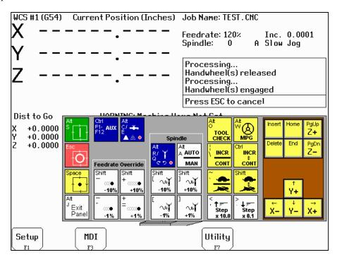
For full functionality of the keyboard jog panel, "Keyboard" must be selected as the console type in the Console Configuration menu.
