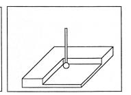
At the end of the probing cycle, the probe will be positioned above the corner at the Z clearance level entered. Press **ESC** to return to the Set Part 0/ Position screen or digitize screen.
