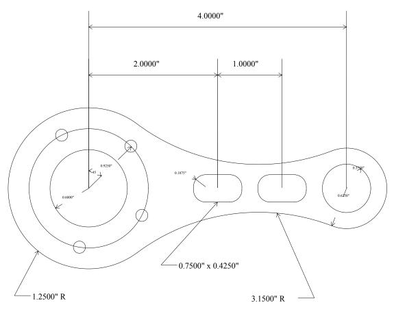
FIG. 1 - Part to be machined.
