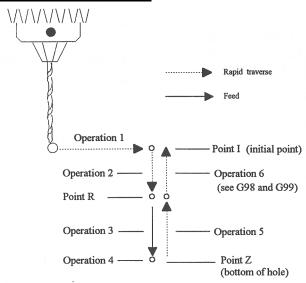
Figure 1. Drilling cycle operation
