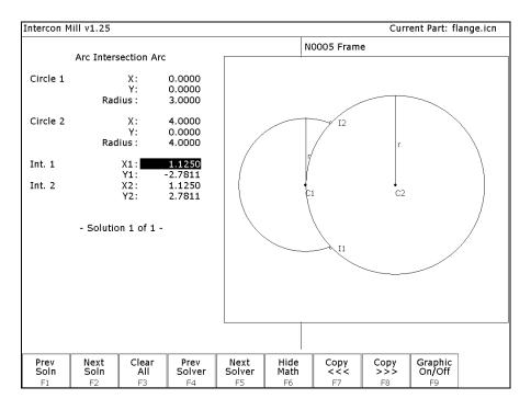
Given the center points (C1 and C2) and the radii (R1 and R2) of two arcs, find the intersection point(s) (I1 and I2) of the arcs.
