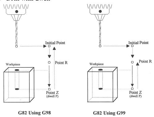
G82 is a general purpose drilling cycle similar to G81. However, G82 includes an optional dwell at the bottom of the hole before retracting the tool. This can make the depth of blind holes more accurate.
