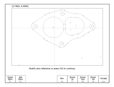
This menu allows you to change the absolute zero reference of the DXF file. The current zero reference appears as a green cross. All other points appear as gray crosses. A new zero reference may be defined by a combination the following methods:
