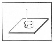
If the Z clearance you entered is too small, the probe will stop and show an error message. Correct the problem by repeating the previous steps. If the approximate diameter you entered is too small, the probe will bounce by 10 percent of its diameter across the top surface until it either finds the correct edge, the additional distance searched is equal to Parameter 16, or a travel limit is reached.
