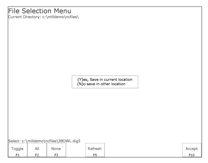
To convert the files and save them in the same directory as the digitized files press Y. To save the files in a different location such as a floppy or USB drive press N, navigate to the desired directory using the file menu, and press F10-Accept to convert and save the files in that location.
