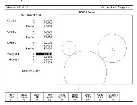
Given the center points (C1 and C2) and radii (R1 and R2) of two arcs and the radius of a third arc, find the center point of the third arc and the tangent points (T1 and T2).
