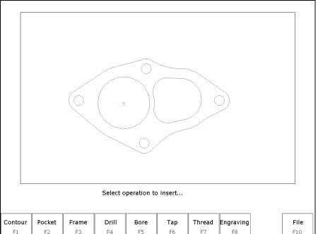
This menu allows you to select the type of Intercon operation you wish to create using geometry from the DXF file.
