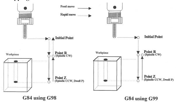
G84 performs right-hand tapping using a floating tap head. The spindle speed and feedrate should be set and the spindle started in the CW direction before issuing G84. By default G84 uses M4 to select spindle CCW (at the bottom of the hole) and M3 to re-select spindle CW (after backing out of the hole). Alternate M functions may be specified by setting parameters 74 (for CCW) and 84 (for CW). See G10 for examples.
