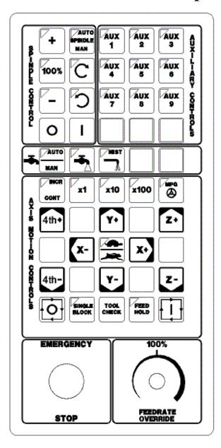
The M-Series operator panel is a sealed membrane keyboard that enables you to control various machine operations and functions. The panel contains momentary membrane switches. The M-Series jog panel can be customized as to the location of various keys. The jog panel displayed in the figure above is representative of a default configuration found on most M-series controls.
