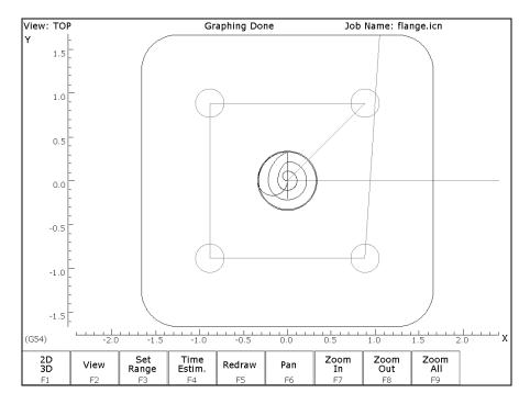
The display will consist of arcs and/or lines that make up the tool path followed. Rapid (G0) moves will appear in Red, linear (G1) and arc (G2, G3) moves will be Yellow, and compensated pass will appear in grey. Canned cycle operations (except the facing cycle) will also display a gray.
