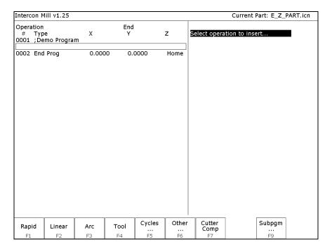
The new operation will be inserted right before the currently highlighted one. The operation types that you can insert are listed across the bottom of the screen.
