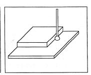
Once the probe has completed its search, it will be positioned above the corner at the Z clearance you specified. Press **ESC** to return to the Set Part 0/ Position screen or digitize screen.
