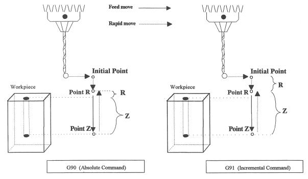
Figure 2: Canned Cycle Absolute and Incremental modes
