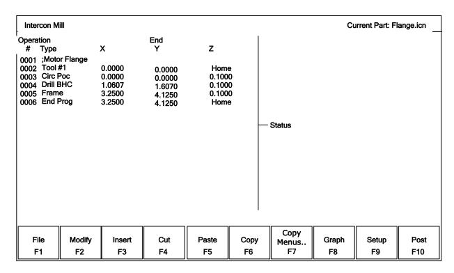
When the part program is displayed, different operations can be navigated and highlighted for additional actions by using the arrow keys, and the HOME, END, PAGE UP and PAGE DOWN keys.
