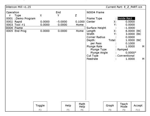
The parameters on the screen correspond to the following dimensions (rectangular frame):
