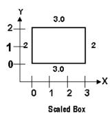
For this G51, the following program lines were scaled 3:1 in the X direction, 2:1 in the Y direction, and 1:1 in the Z direction. If no scale factor is specified, the default is 1:1 for all axes.
