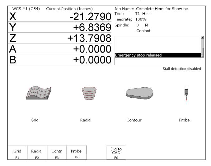
The Digitize feature of CNC10 is used to digitize a rectangular surface area (grid), an inside circular bore area (radial), or a contour. The digitizing process creates a file with M & G codes that represent the digitized surface. If the digitizing probe tip is chosen to match the milling cutter size, the digitized file can be loaded and run to produce an exact copy of the digitized part.
