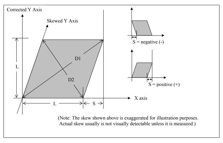
If you have trouble directly measuring S, you can calculate it by measuring the diagonals D1 and D2, and then using the following formula:
